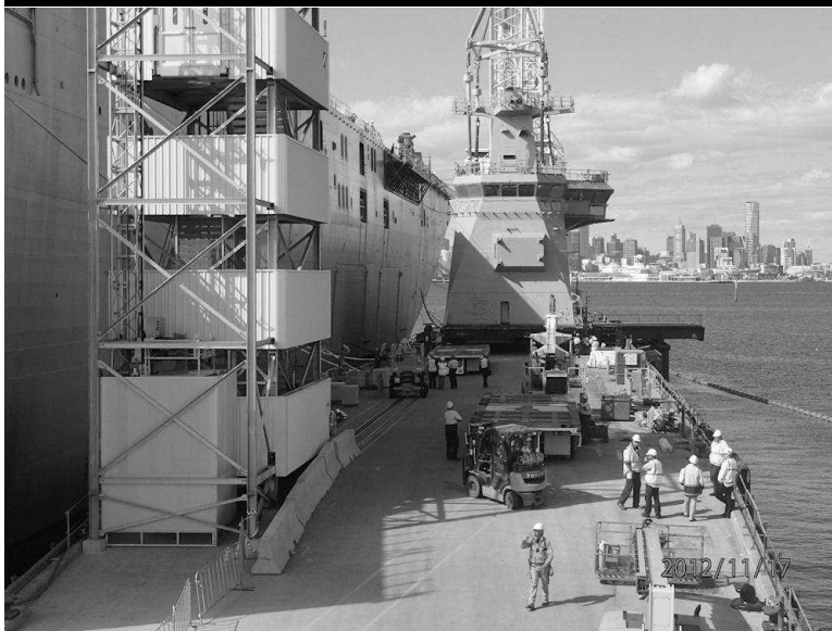
ABOVE Superstructure block ready to be lifted to the deck.
